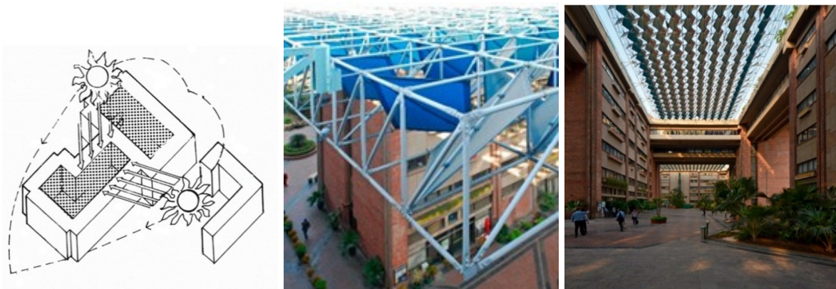
Figure 10: Shading of the internal courtyard in the Indian Habitat Centre (Source: Sanyam Bagha, Gaurav Raheja)
